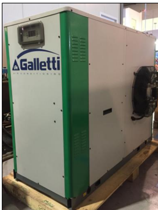
Figure 4.5 Dual Source heat pump for high temperatures (prototype #3)
