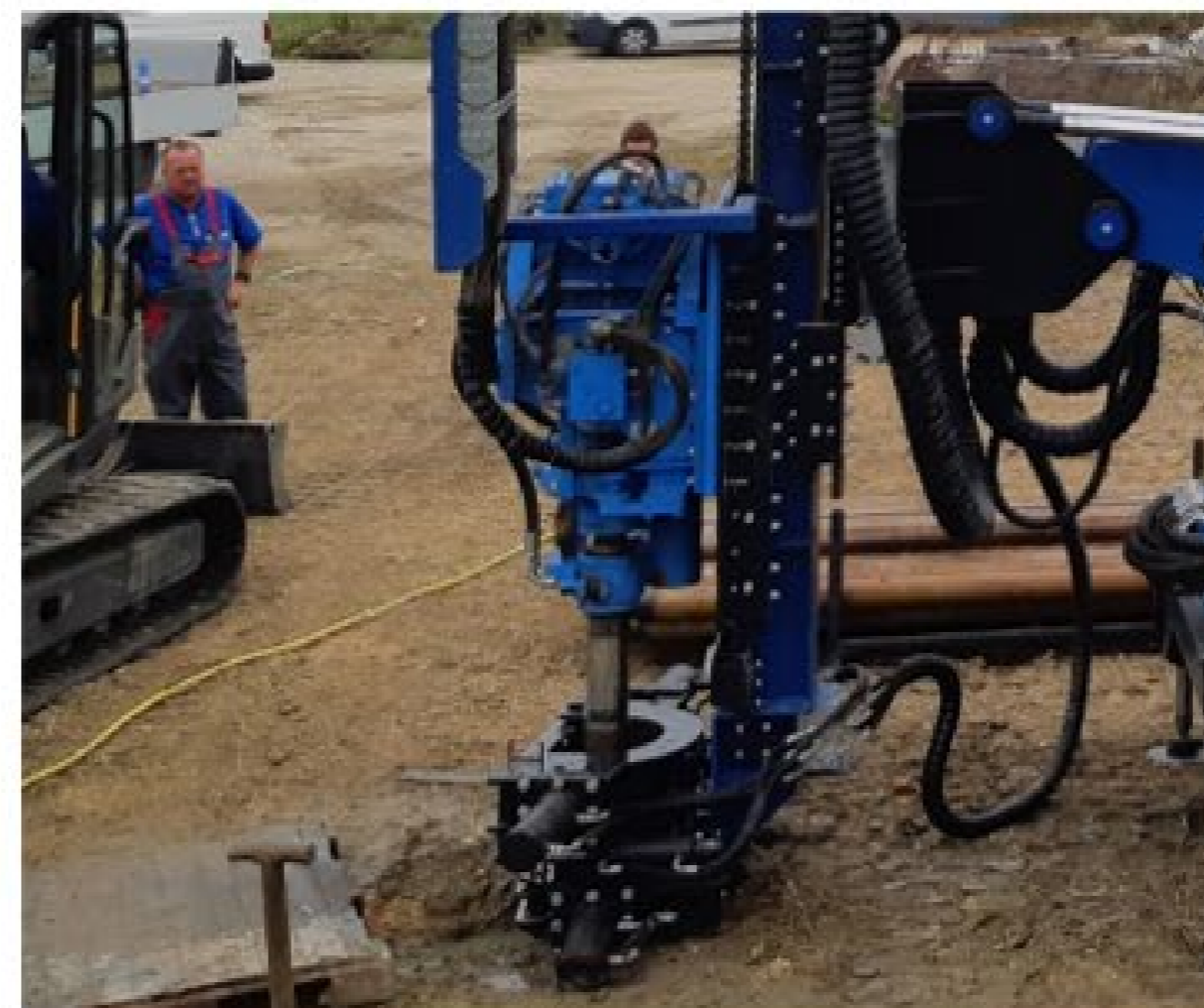
Drilling with water flushing in clay, sand, gravel
