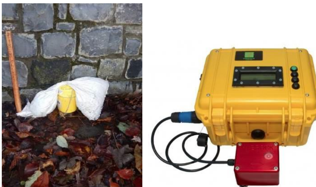
Figure 3.2 Example of improved coupling using sandbag b) Vibrock V901 instrument and single geophone (red)
