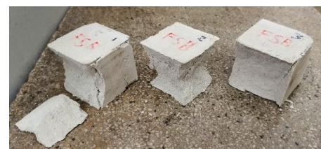
Fig. 7. Average cubic compressive strengths of the grouts plus or minus one standard deviation (a), RF grout samples before compression tests (b), and FSB samples after testing presenting the typical hourglass failure surface (c).
