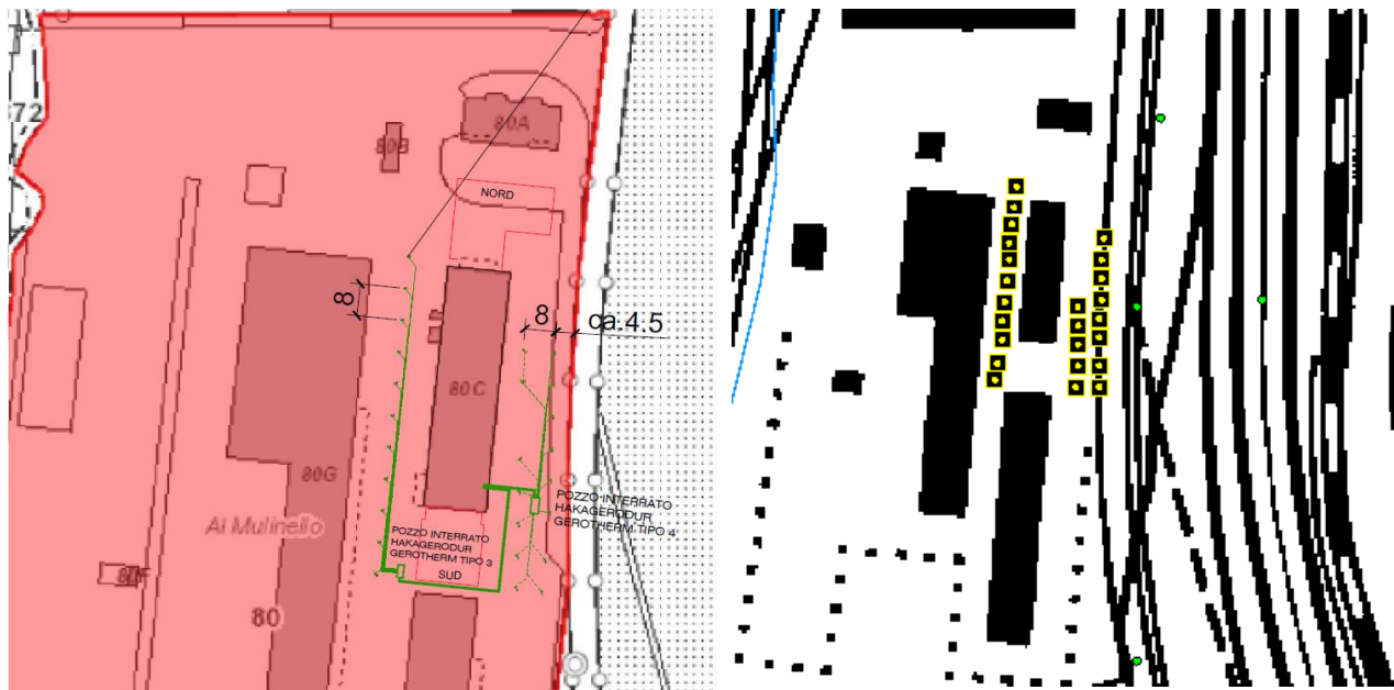
Figure 3: Disposition of drilling on the project plan (left), and of the cantonal database (right). The scheme with the BHE disposition on the field, at a minimum distance of 4.5m from the border (5% of 90m depth). A screenshot of the BHE recorded on the cantonal database is also shown (this information is available for the public, and during years).
