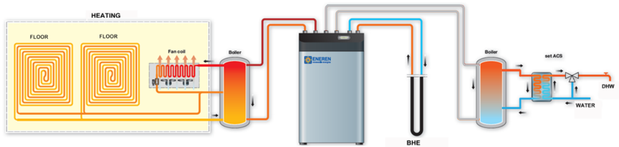
Figure 16: Layout of ON-OFF heat pump solution
