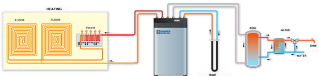
Figure 23: System layout with multi-function heat pump
