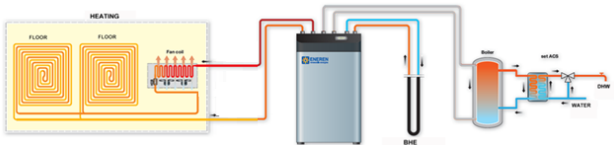
Figure 22: System layout with Inverter heat pump
